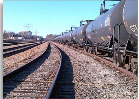
Rail shipments of petroleum crude oil typically consist of unit trains of over 100 tank cars, with each tank car containing approximately 30,000 gallons of crude oil.
