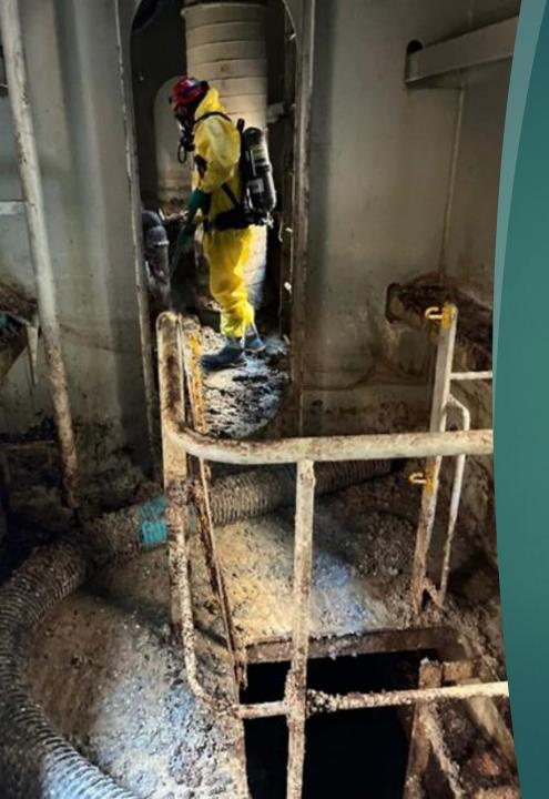
Underdeck Passageway at Tier 04 Level (second from bottom). Shoveling sludge/soybean mixture to bottom of cargo hold and towards pump. Level B primarily for high H2S readings.
