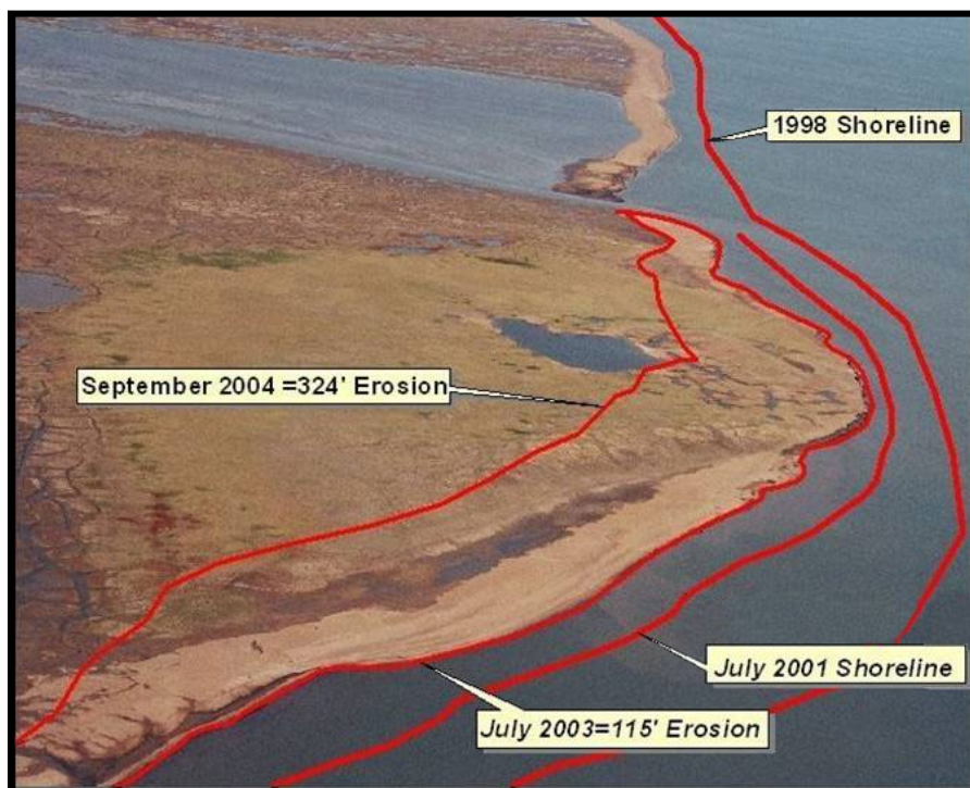
Figure 9-1: Drill Site Erosion
